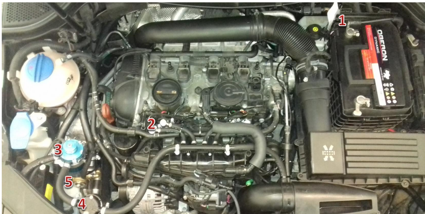
1-sterownik/ECU Zenit Direct, 2-wtryskiwacze gazu/gas injectors, 3-reduktor/reducer, 4-filtr fazy lotnej/gas phase filter, 5-elektrozawór z filtrem fazy ciekłej/electrovalve with liquid gas phase filter
